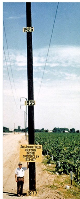
Figure 5.2: An Image of Maximum Subsidence in the San Joaquin Valley from 1925 to 1977. 45
